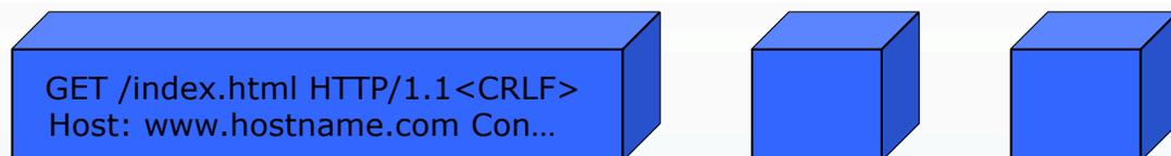
**HTTP Message's data stream is chopped up into chunks small enough to fit in a TCP segment**
